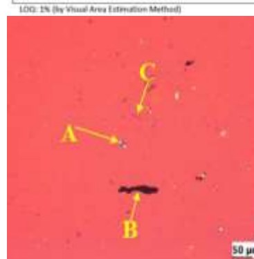
Figure 6. PLM image of particles in sample "200-2022-04220053" A: Starch B: Rust/Metal Dust C: Skin Fragment
