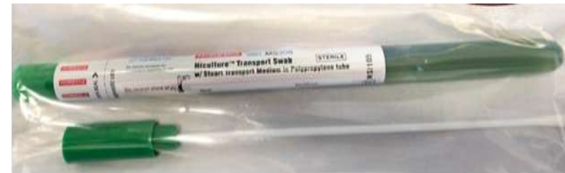
HiCulture Swab used with 3M phosphate buffer as collection solvent
